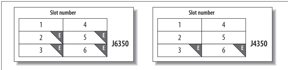
Figure 2-3. J6350 and J4350 PIM slot numbers
